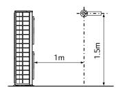
These figures assume the following operating conditions: Equivalent piping length: 7.5m Level difference: 0m
