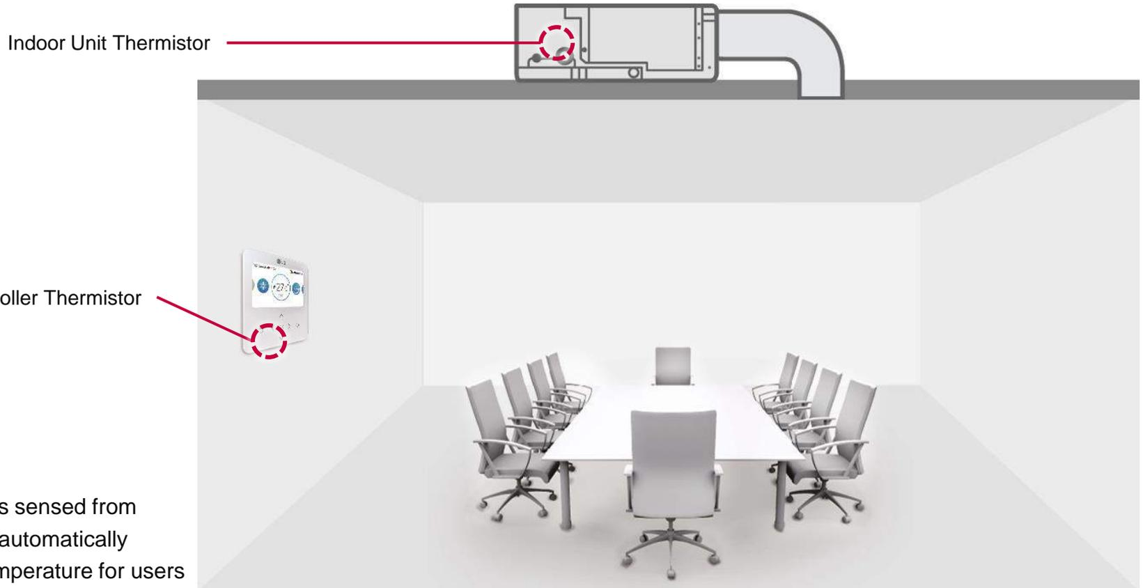
Compares temperatures sensed from different positions, and automatically selects the optimum temperature for users
